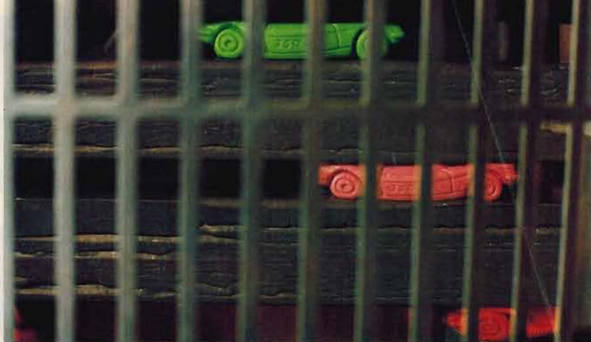
Caltech's remarkable interferometer has some unremarkable components: tiny rubber cars help cushion the system's suspended masses against tremors.
