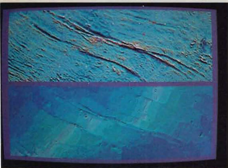
Satellite gravity map (top) filled in gaps that remained from bathymetric surveys from ships. Bathymetric map (middle) shows finer detail but not fractures beneath sediment; gravity map does. Close-up of the Eltanin Fracture Zone
