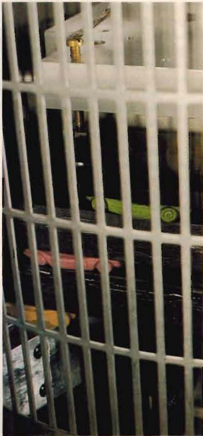
Logic and ingenuity are essential in solving sensitive design problems, but a sense of humor can't hurt. All three are evident in the Caltech solution to the problem of eliminating extraneous vibrations in their system: The frames that hold the masses are stabilized with alternating layers of rubber toy Mercedes Benzes and dune buggies.
